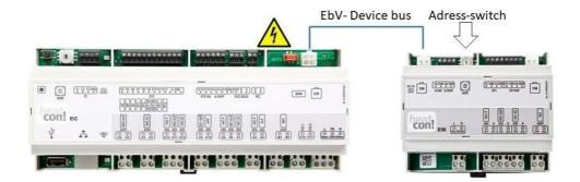
The heatcon! EM is an expansion for the inputs and outputs of a heatcon! EC inside the system, as shown in the technical data.
