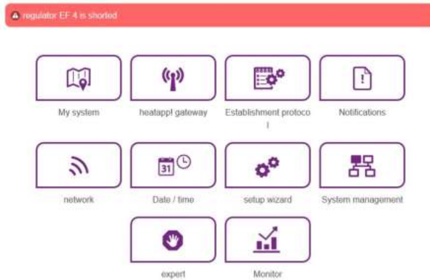
Fig. 88: Typical fault message on the PC user interface
