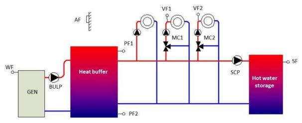
Fig. 75: Buffer charge control with heating circuit and hot water requests
