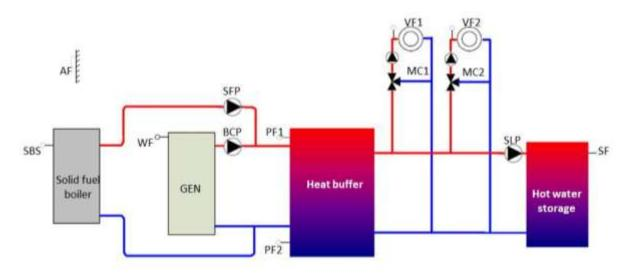
Buffer charge control (BULP) for heating circuit and hot water with solid fuel regulation
