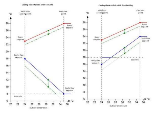
Fig. 64: Connection room setpoint temperature  $\Leftrightarrow$  flow temperature
