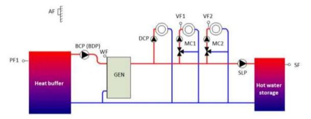
*Fig. 82: Buffer discharge control type 2 on heat generator*
