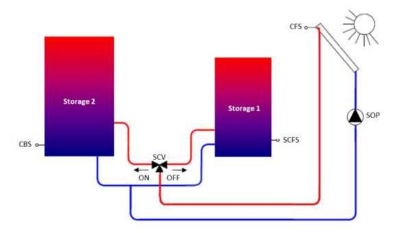
*Fig. 83: Double buffer system of a solar thermal system (example)*
