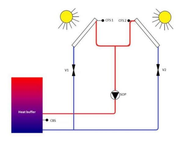
*Fig.* 84: Solar - double collector array (example)
