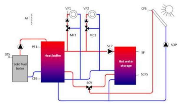
Solid fuel regulation with buffer storage solar system with solar charge valve
