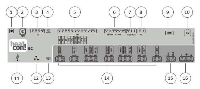
Fig. 26: heatcon! EC - connection assignment
