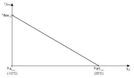
Fig. 69: Calculation of the advanced switch-on time
