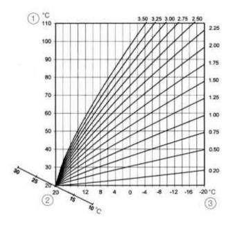
Fig. 67: Heating Characteristic Curve
