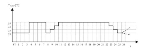
Fig. 72: Time sequence - functional heating with subsequent floor covering heating
