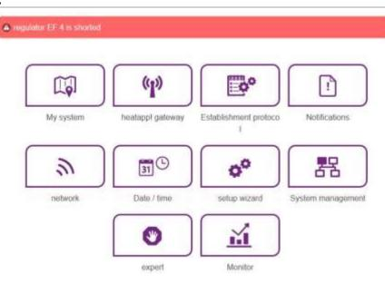
Fig. 88: Typical fault message on the PC user interface
