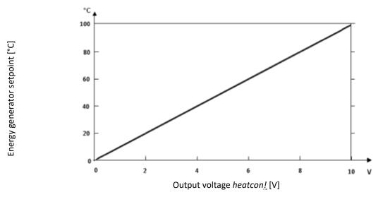
Fig. 55: Performance chart with adaptation to the energy generator
