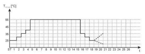
Fig. 71: Time sequence - floor covering heating
