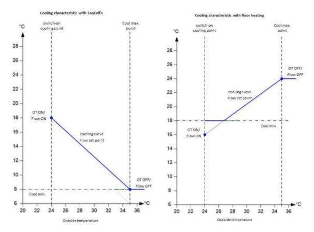
Fig. 62: Cooling curve Point 1 of curve (OT-On / FT-On):<:
