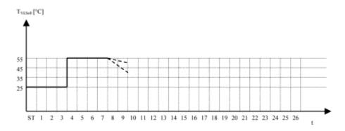
Fig. 70: Time sequence - functional heating
