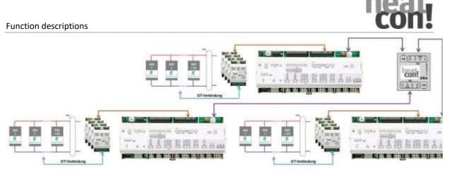
Fig. 58: OpenTherm cascade fully equipped
