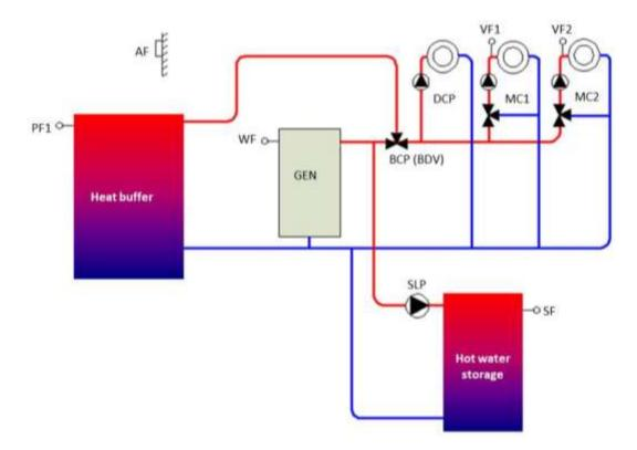
Fig. 81: Buffer discharge control on HC
