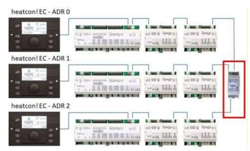
Fig. 56: Connection of several heatcon! EC with heatcon! EM-GBA
