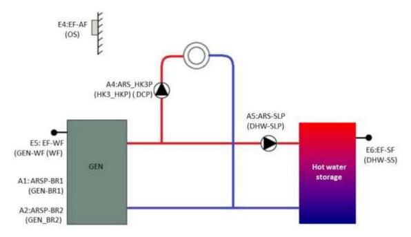
Fig. 95 Single or two-stage GEN with unmixed heating circuit and DHW
