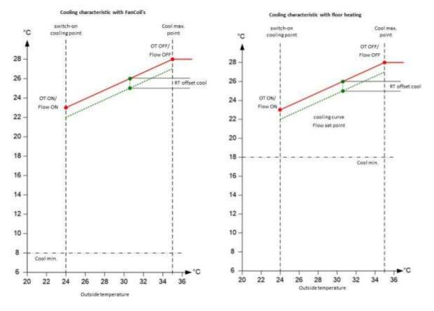
Fig. 63: Calculating room setpoint temperature
