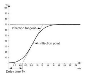
*Fig. 60: Heating characteristic curve (example)*
