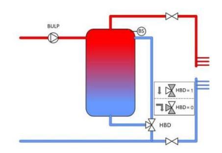
Fig. 74: Example hydraulic scheme, Hydraulic buffer discharge HBD
