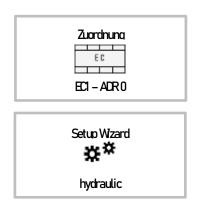
After switching on the power supply, the assignment of the MMI to the heatcon! EC starts. By default EC1 with address 0 is selected. After the assignment, the setup wizard starts automatically in heatcon! MMI.
