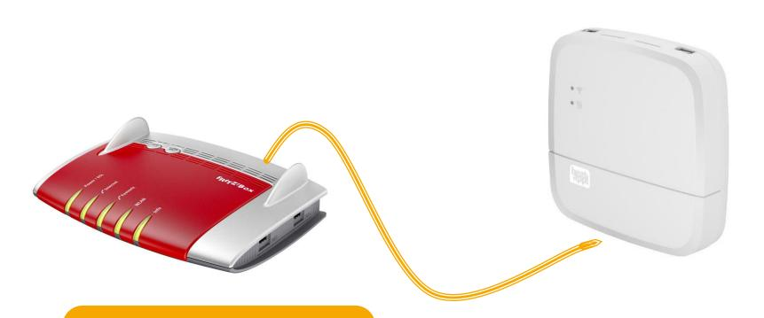
Primary connection via LAN cable with RJ45 plugs between heatapp! base and customer's router.
