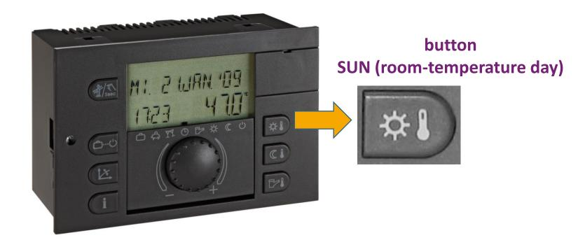
Press button SUN short will guide you to "room temperature day". This value is not an absolute value, but an offset in relation to the "room temperature day" which is used in the cycle time
