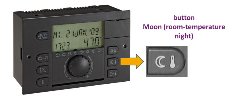
Press button MOON 3 sec. and temporary mode "ABSENSE UNTIL" will appear. By pressing the button MOON for a short time the ABSENSE MODE will be activated.
