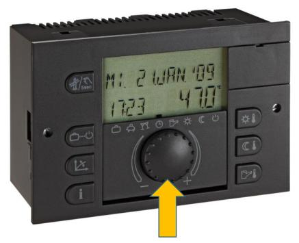
central button for most settings is the central turn-push button "flashing" display can be changed by turning the central button By pressing the central button 3 sec display will jump in menu selection Then pressing the central button short display will jump into specific menu and parameters Save settings by pressing the central button short.
