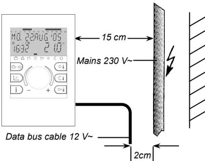
Fig. 1: Minimum distance for cable installations
