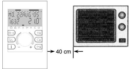
Fig. 2: Minimum distance to other electric supply
