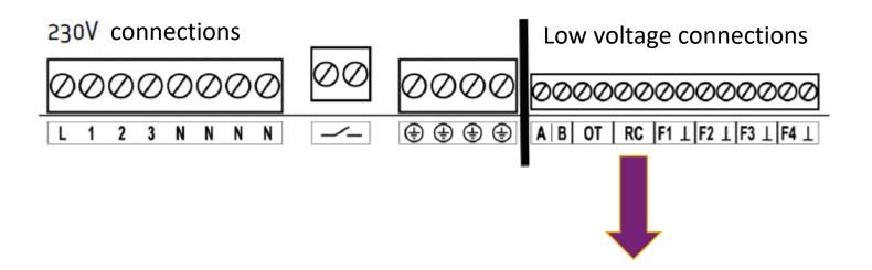
A room control / remote control CETA-RC is connected to the RC terminals.
