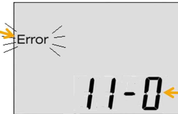
The error code is displayed alternately with the basic display.
