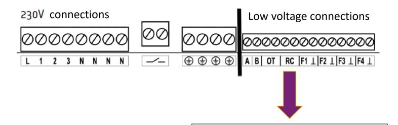
A remote control CETA-RC is connected to the RC terminals.
